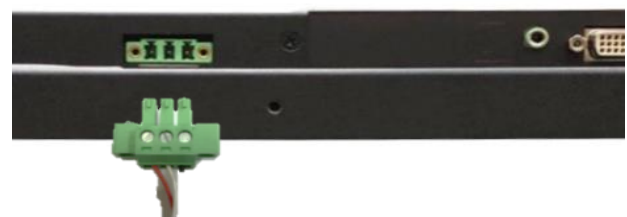
Option 2 / Phoenix Terminal Block/Plug
