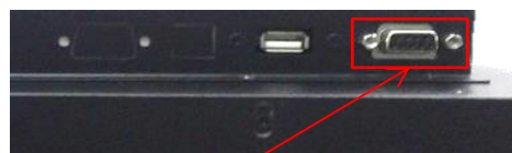
Software Control via RS232 interface.
