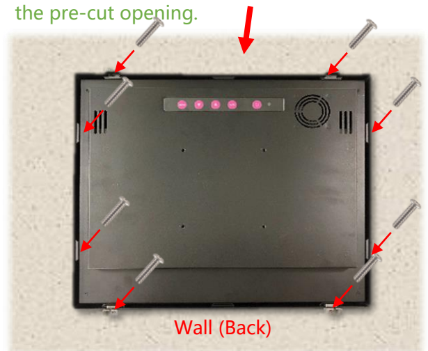
Step 3: Attach the clips from the back and secure with screws. (Up to 8 clips can be installed as needed or per positional limitations.)
